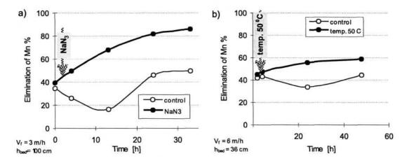
Fig. 2. Efficiency of manganese elimination during the I-st stage filtration on mature sand filter before and after inhibiting microbial activity by intoxicating the bed with  $NaN_3$  (a) and by treating the bed with high temperature (b).
