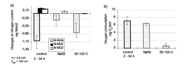
Fig. 3. Changes of contents of various forms of mineral nitrogen (a) and oxygen consumption (b) during the I-st stage filtration on the mature sand filter before and after inhibiting microbial activity.
