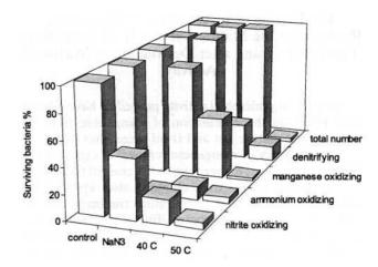
Fig. 1. The percentage share of bacteria surviving on the sand bed after intoxication with 15 mM  $NaN_3$  and after treatment at 40°C and 50°C.
