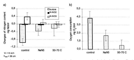
Fig. 5 Changes of contents of various forms of mineral nitrogen (a) and oxygen consumption (b) during the II-nd stage filtration on the mature sand filter before and after inhibiting microbial activity.
